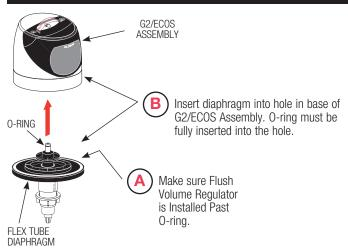
To facilitate installation, wet the diaphragm assembly (on top or completely).
