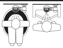
3. When the user steps away, the loss of reflected light initiates an electrical "one-time" signal that activates the flushing cycle to flush the fixture (1 second for urinal, 3 seconds for closet). The Circuit automatically resets and is ready for the next
