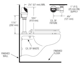
When installing the G2/ECOS in a handicap stall:
